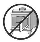
The viewing door must be closed and latched during operation.
