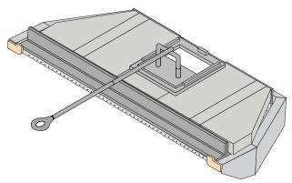
2. Unscrew and remove the bypass damper rod and ring form the damper yoke.
