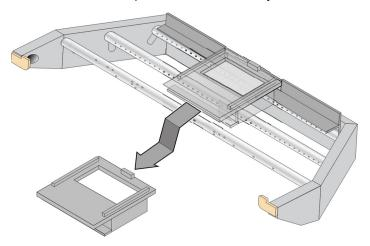
10. Remove the rear baffle support by lifting it straight up until it can clear the air tubes. Move it forward and remove it from the insert.
