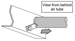
With the bolt loosened the air tube can be slid out of the air channel.
