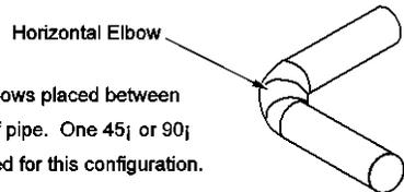
Horizontal elbows are elbows placed between two horizontal sections of pipe. One 45° or 90° horizontal elbow is allowed for this configuration.
