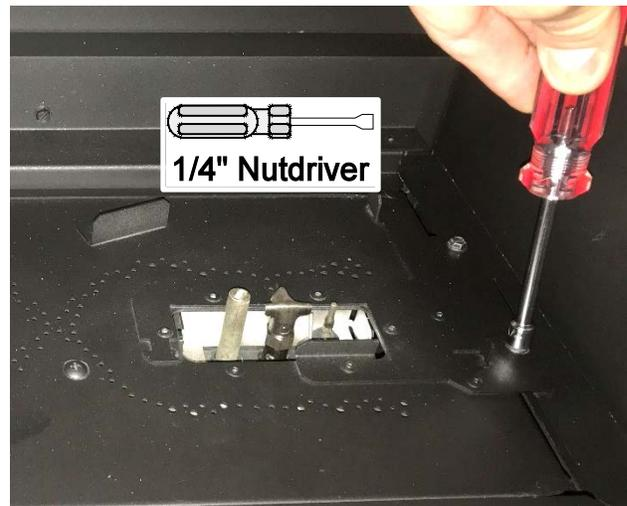
Remove the burner and place it aside.
