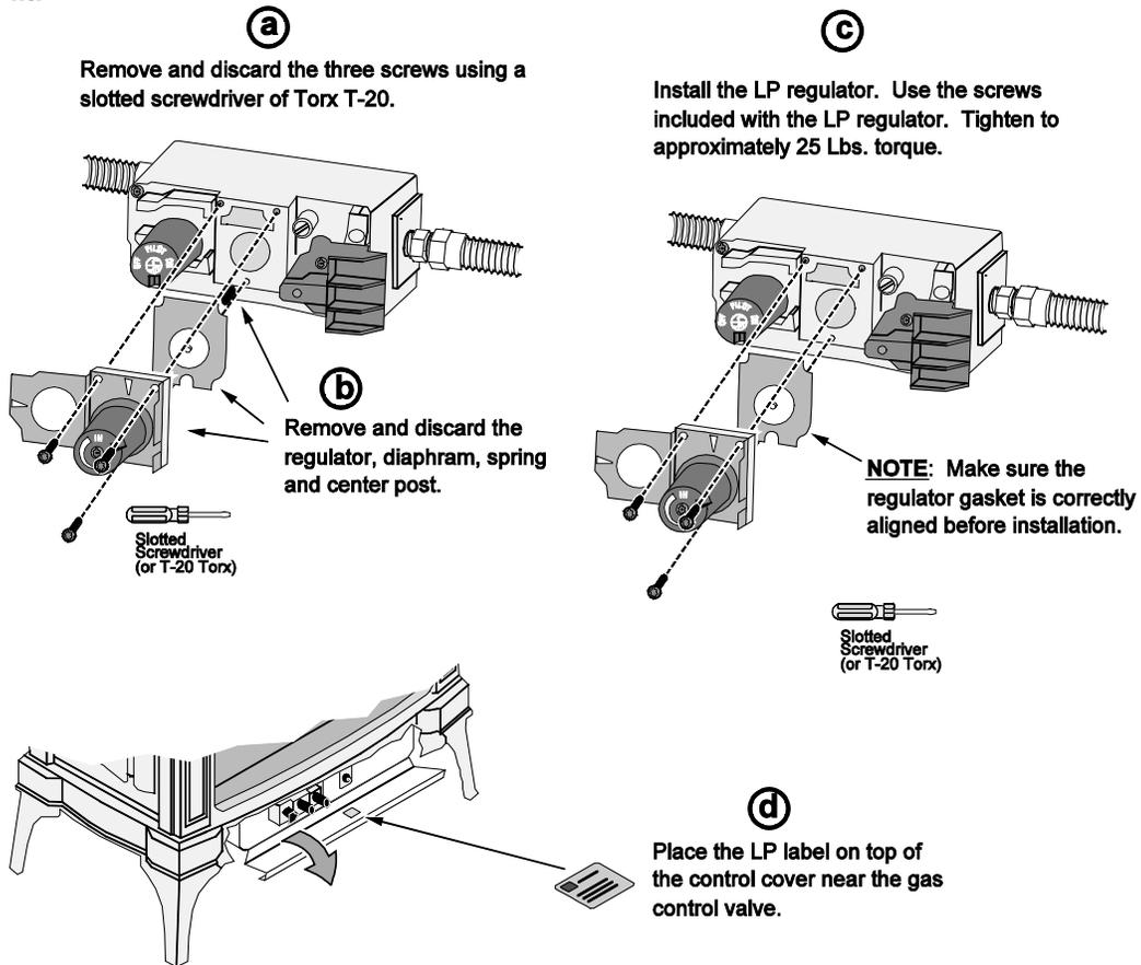
Make the gas line connection, bleed the gas line (if applicable), start the heater and thoroughly leak-test all gas connections and the gas control valve.
