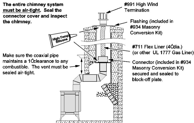
**\*CAUTION:** This vent configuration is not covered under the appliance safety standard (ANSI Z21.88 CSA 2.33) used in the safety certification of this appliance, however, this method has been tested by Travis Industries and it has been determined to be safe following the instructions above. Before installing the appliance using this method, contact the Authority Having Jurisdiction to determine if this installation is acceptable in your area.
