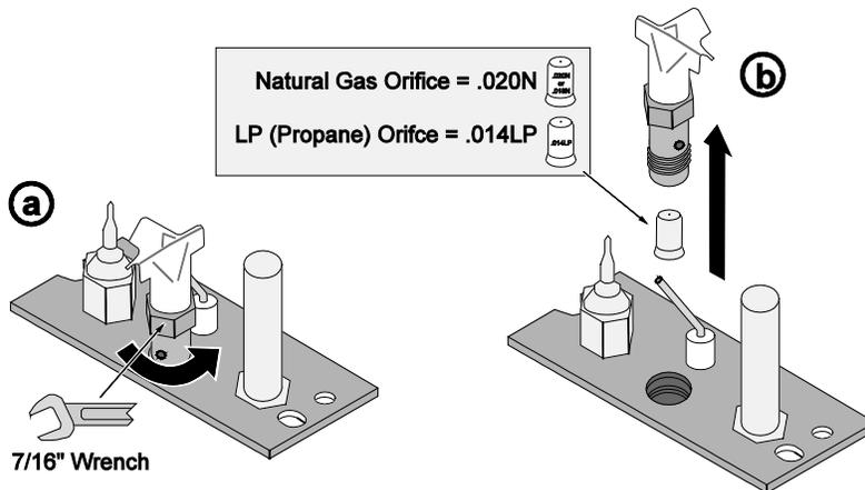
Remove the burner orifice and discard. Install the LP (propane) orifice.
