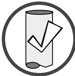
Inspect the chimney connector and chimney at least twice monthly and clean if necessary. Creosote may build up and cause a house fire.
