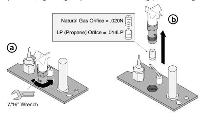
6. Remove the burner orifice and discard. Install the LP (propane) orifice.
