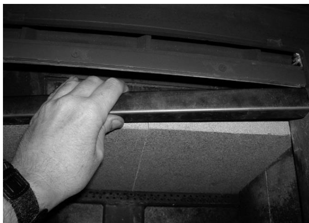
Figure 16 - Removing/Replacing the Baffle for Inspection
