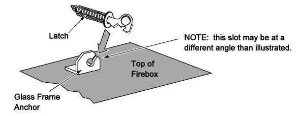
Note how the washer on the latch fits behind the flange on the glass frame anchor.
