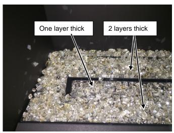
4 Make sure the rear and end air channels are free of crushed glass. Use a screwdriver to clear this area. Make sure the glass is only 1 layer deep on the burner.
