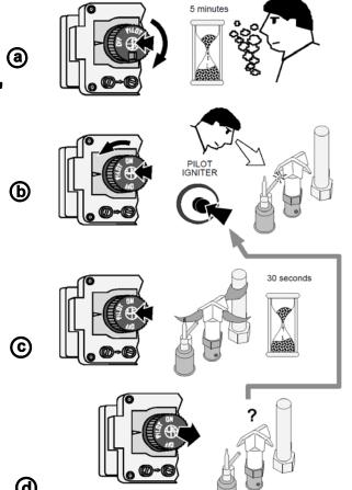
With the pilot lit, the heater can be operated using the normal controls. Make sure to return the heater to the correct configuration before proceeding (replace logs, glass, barrier screen, if applicable).
