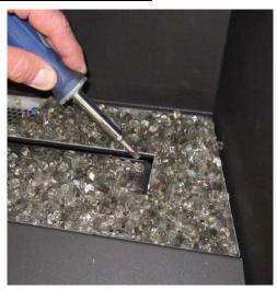
5 Remove the pilot shield to uncover the pilot once you are finished placing the glass.
