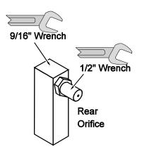
Use a 9/16" wrench to secure the manifold while removing the orifice with a 1/2" wrench.
