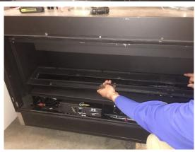
3. Remove both burners. Each is held in place with 6 screws (1/4" nutdriver).
