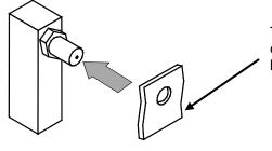
The longer portion of the gasket should be at the bottom.
