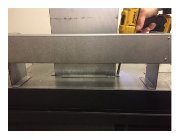
4 Remove the (4) screws from each of the (2) header shields (keep the screws for reinstallation). Turn each of the shields over endwise and secure them back into place using the screws you just removed. The bent edge of the shields should be facing upward and toward the back of the fireplace (see illustration below).
