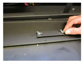
Align the two holes on the bottom of the receiver assembly with the studs and secure the assembly to the bracket using the two wing nuts removed in the previous step.
