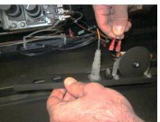
4 Remove the switch from the dashboard by depressing the tabs on the top and the bottom of the switch housing while pressing the back of the switch forward through the hole in the dashboard. Replace the switch with the included switch blank (see pictures below).
