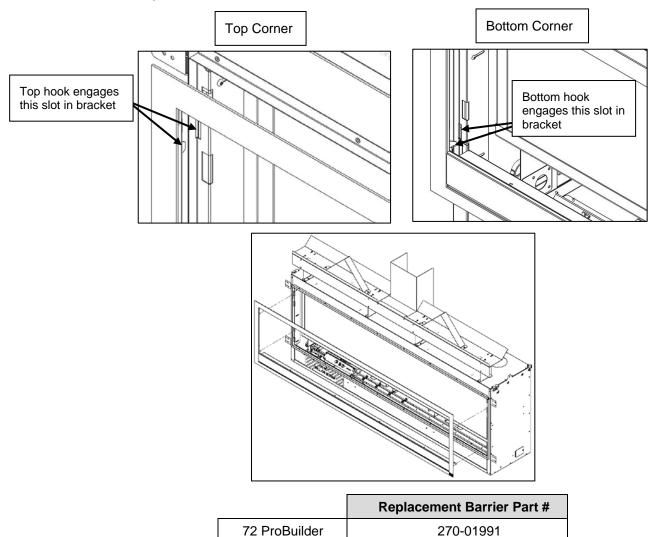
2. Remove the glass frame following the directions below.
