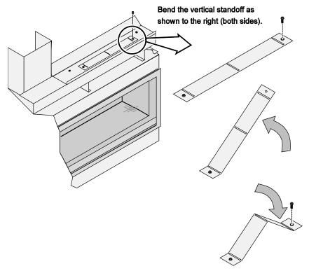
6 When finished the fireplace should be configured like the picture below.
