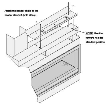
The (2) header standoffs are screwed down flat to front edge of the top of the shields. On each standoff, remove the screw that is closest to the outside edge of the fireplace (keep screw for reinstallation). Bend the legs at the perforations as shown below and attach the foot of the standoff to the top of the fireplace using the screw removed earlier in this step.
