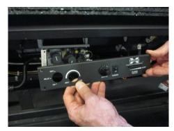
**NOTE** There should be enough slack in the attached wires to lower the dashboard to the floor. Make sure not to damage any off the attached wires.
