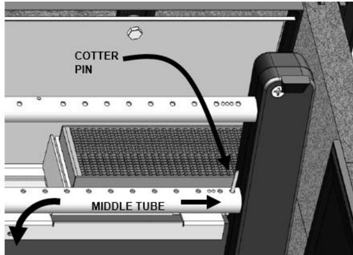
**Figure 19 – Removing the Middle Air Tube**
