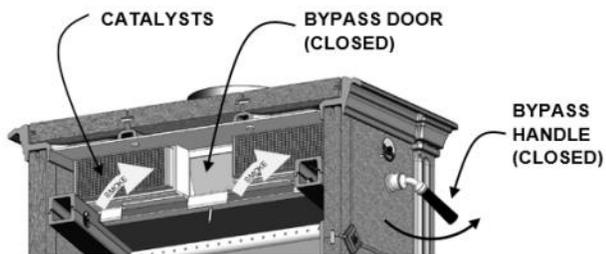
Figure 14 – Bypass Closed
