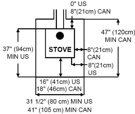
When installed on a combustible floor, non-combustible floor protection is required to cover the area beneath the heater, and extend at least 16" (41cm) [18" (46cm) CAN] to the front and 8" (21cm) beyond each side of the fuel loading and ash removal openings [side of stove in CAN], the floor protection must extend under the flue connector and extend 2" beyond each side of pipe.
