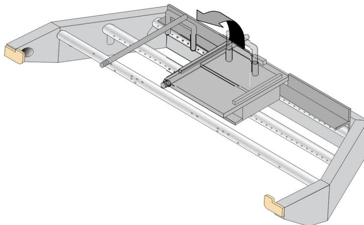
8. Remove the bypass slider by sliding it forward, off of the bypass slide plate and remove it from the insert.
