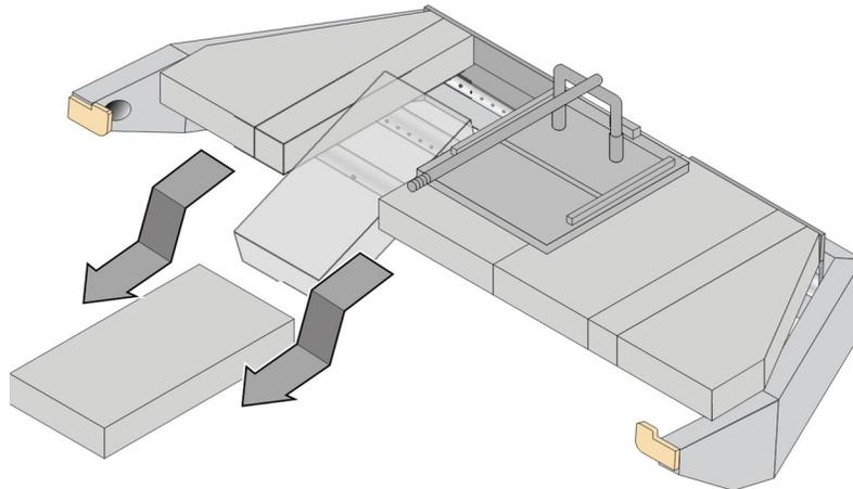
7. The yoke can now be removed by lifting it upward until the yoke legs are free from the cups on the bypass slider.
