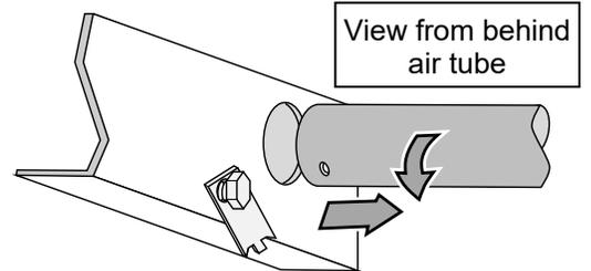
The pin will then disengage from the air tube (you may wish to rotate the tube slightly).
