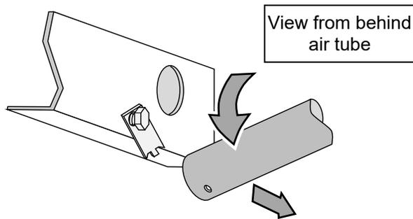
Pivot the air tube downwards and slide it out of the air channel on the opposite side.
