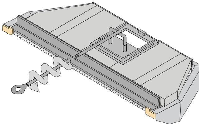
3. Remove front brick retainer by pushing up the front edge and sliding it over the retainer tabs. Slide the support forward until it is out from under the baffle bricks. Maneuver the baffle support out through the door opening.
