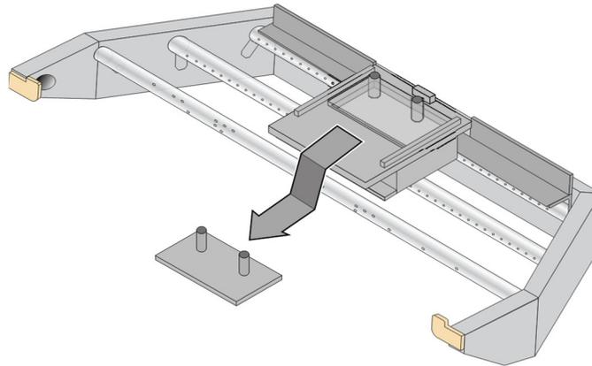
9. The bypass slide plate can then be slid forward and removed from the insert.
