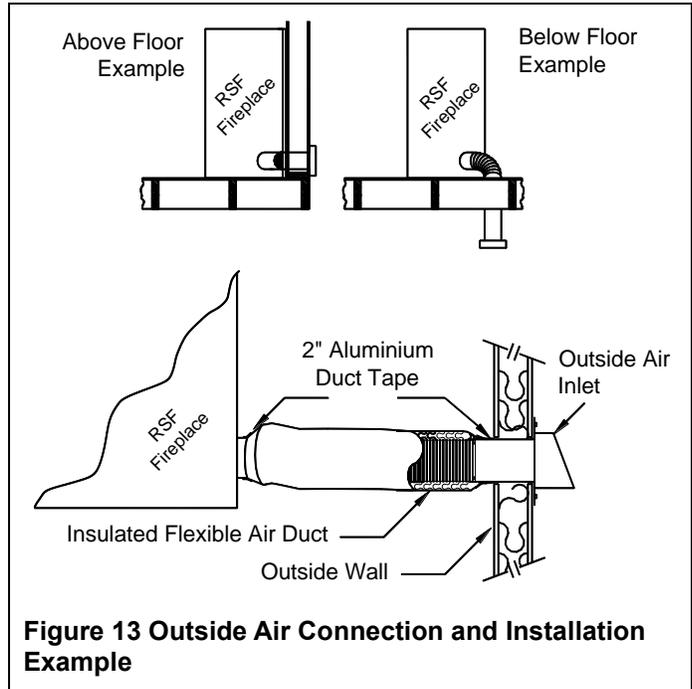
**Figure 13 Outside Air Connection and Installation Example**
