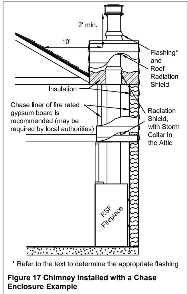
**Figure 17 Chimney Installed with a Chase Enclosure Example**
