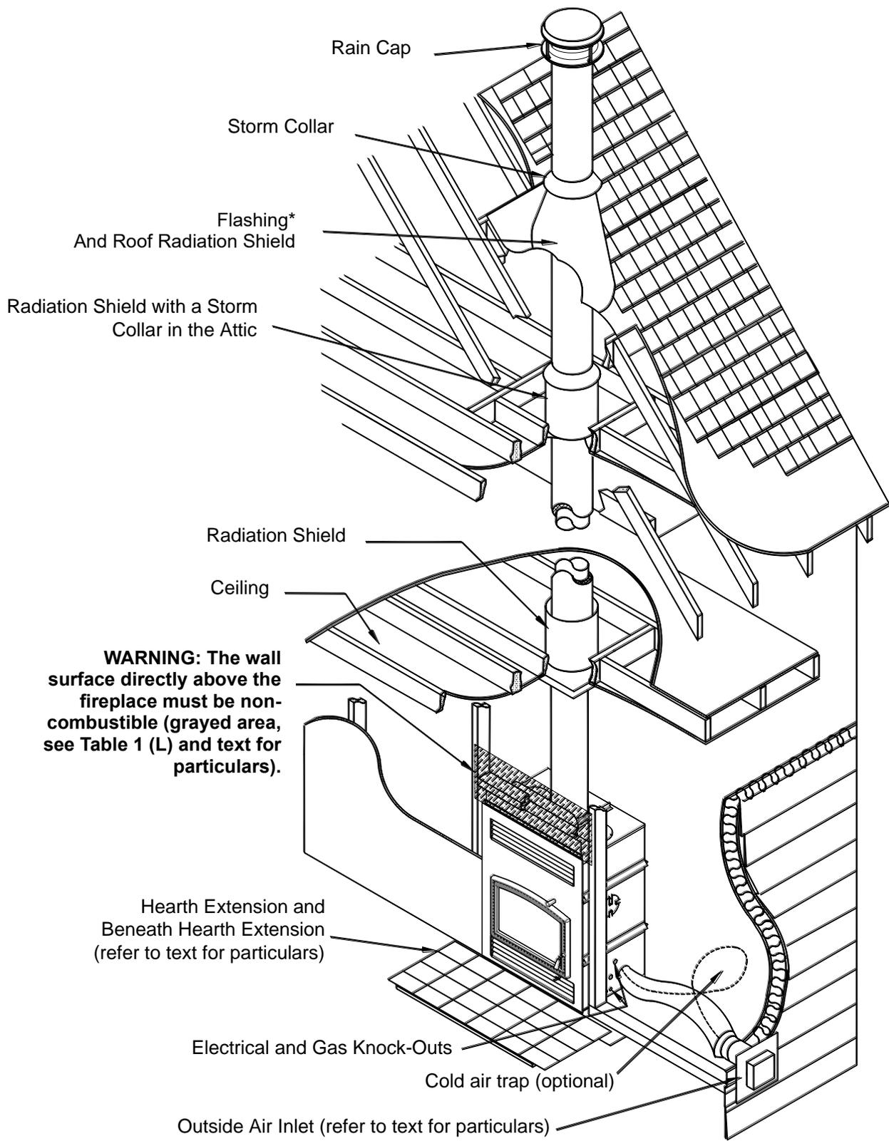
**WARNING:** The wall surface directly above the fireplace must be non-combustible (grayed area, see Table 1 (L) and text for particulars).
