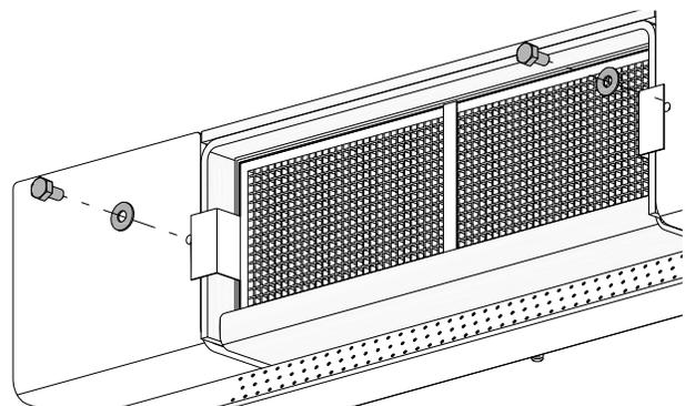
Wrap the new catalyst on all sides with the catalyst gasket. Enough gasket is supplied to wrap the catalyst with two layers of the gasket material. Carefully insert the catalyst and catalyst support plate into the opening and reinsert all four screws that hold it in place. The catalyst gasket expands as it is heated; so, it is normal for the gasket to have some small gaps after being inserted. As the gasket expands, the spaces will be filled.
