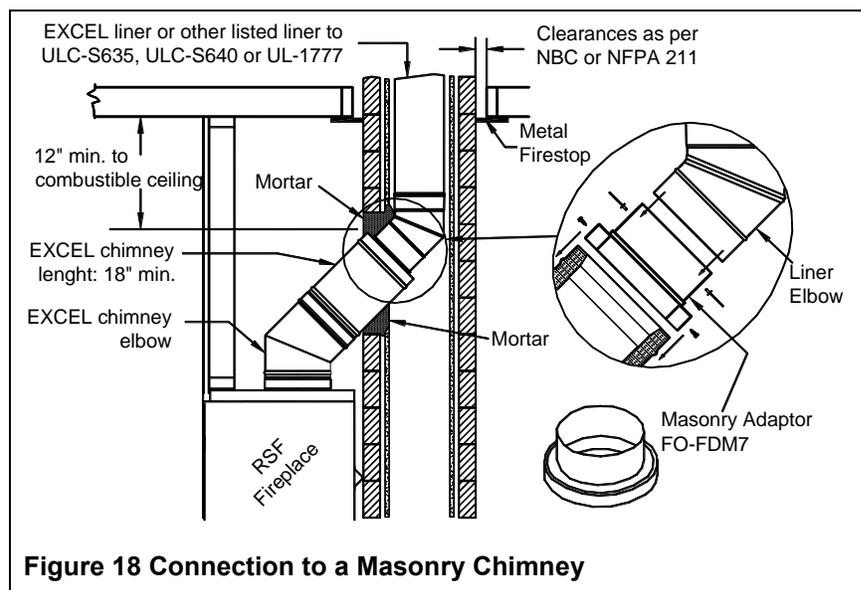
**Figure 18 Connection to a Masonry Chimney**
