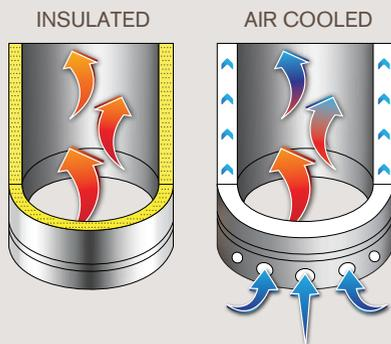
Most fireplaces use air cooled chimneys which circulate cold air past the inner flue to reduce the temperature. A cold flue makes establishing a draft difficult and increases the formation of creosote in cold weather.
