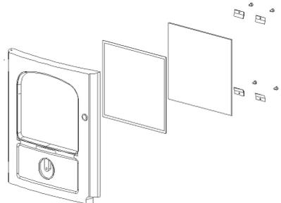
1. Lift the door off its hinges and place face-down on a sheet of cardboards or other non-abrasive fabric. The door is removed by loosening the 2 screws with a hexagon box wrench by the hinges.
