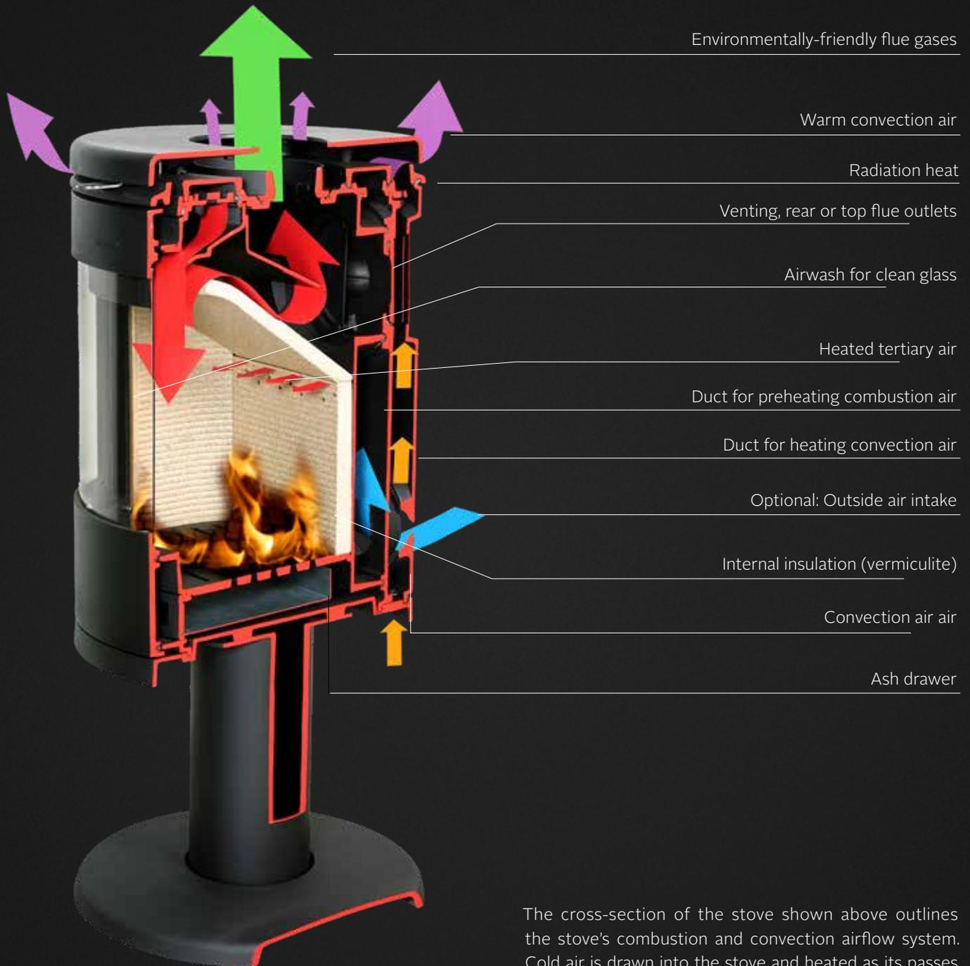
The cross-section of the stove shown above outlines the stove's combustion and convection airflow system. Cold air is drawn into the stove and heated as it passes through the cast iron channels (the heated air washes the glass keeping it clean, clear and free from soot). The hot air also provides perfectly heated combustion air (in addition the heated tertiary air aids secondary combustion of any smoke and gasses, increasing efficiency and reducing the environmental impact).
