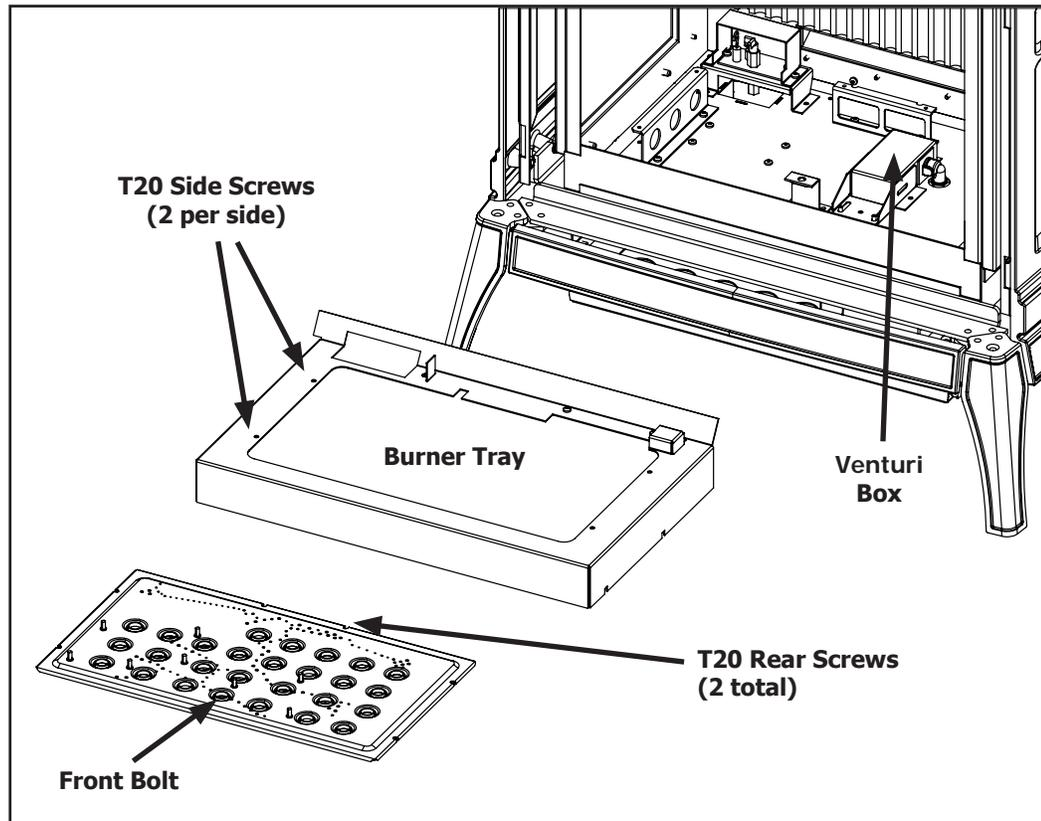
Figure 23. Burner Removal
