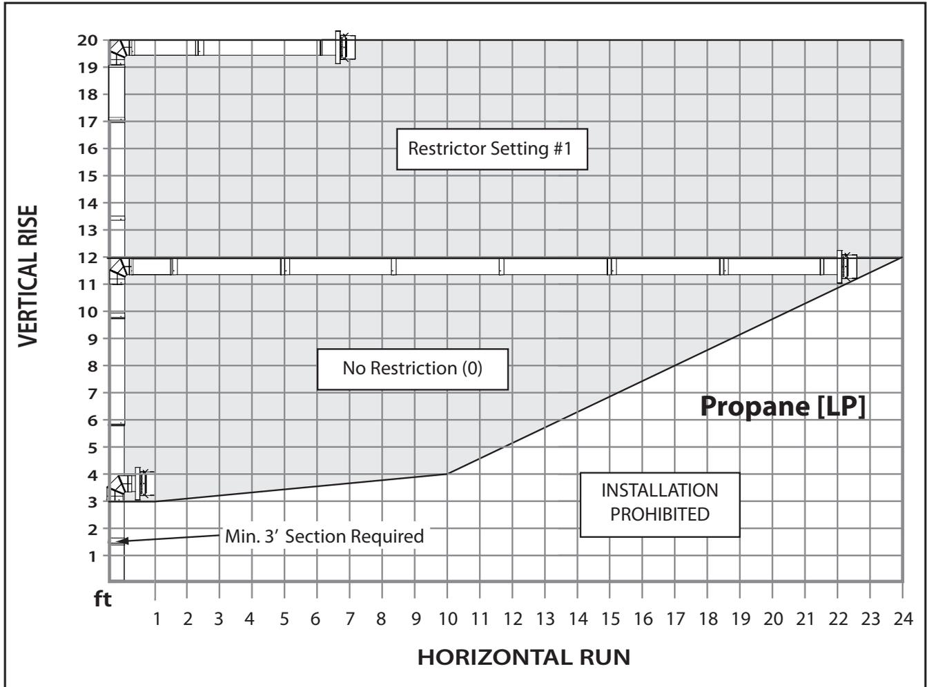
Figure 34: Horizontal Termination - 1 Elbow [LP]
