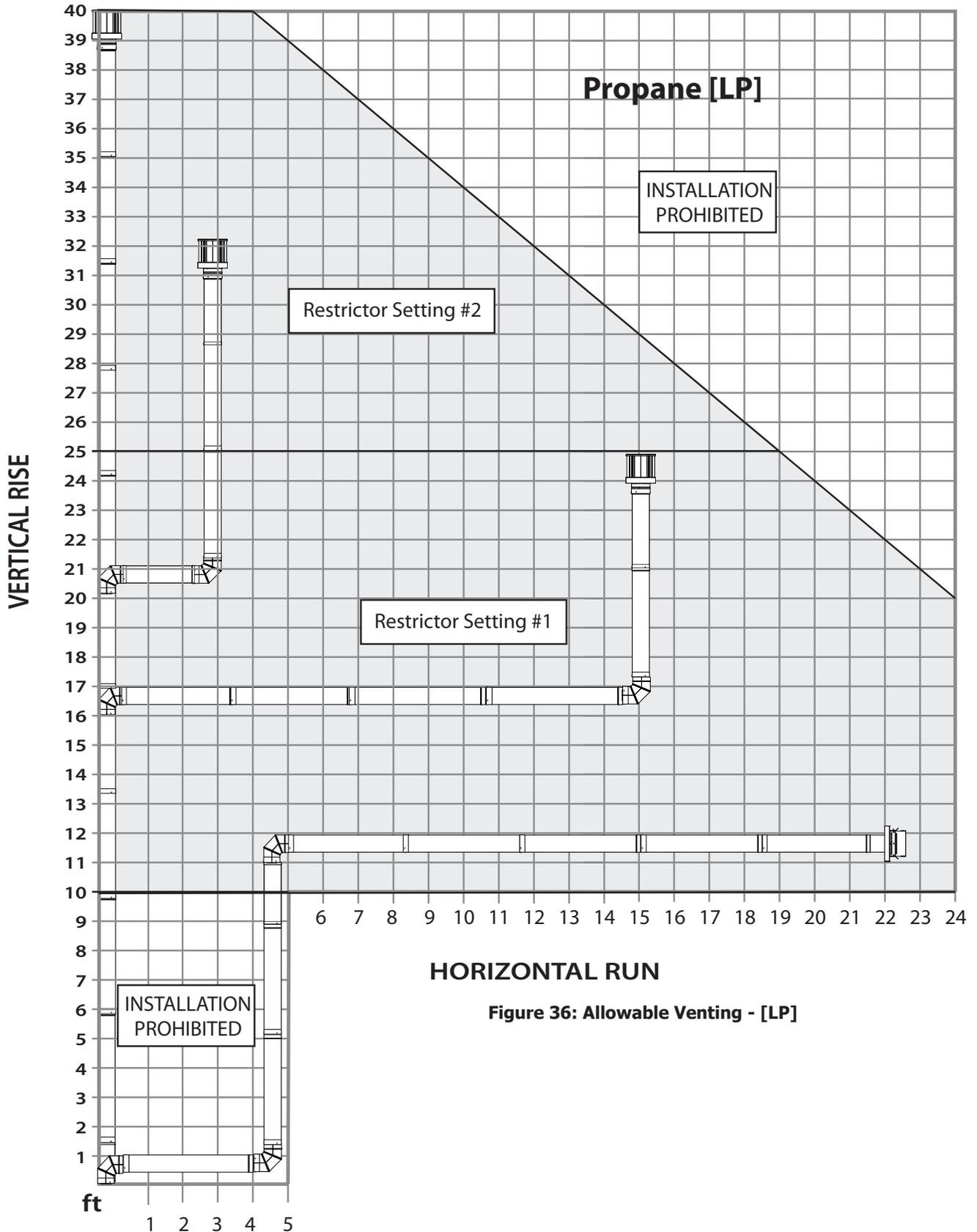
Figure 36: Allowable Venting - [LP]
