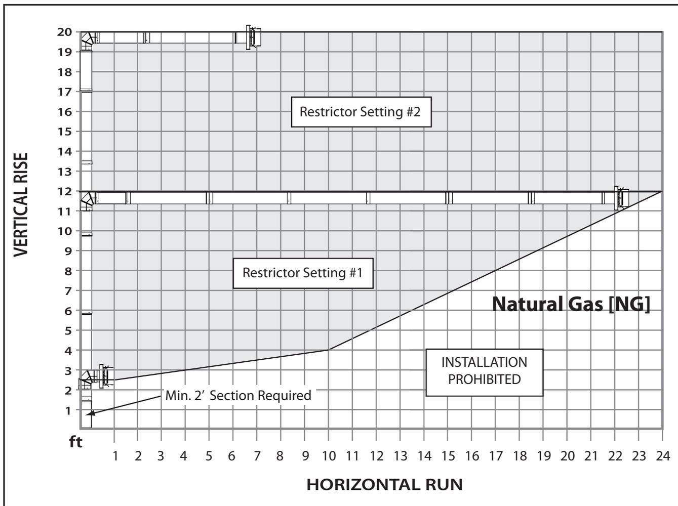
Figure 33: Horizontal Termination - 1 Elbow [NG]
