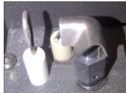
Figure 25 Proper Pilot Position
