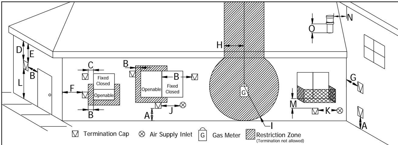
**Figure 30. Vent Termination Restrictions, refer to Table 5.**
