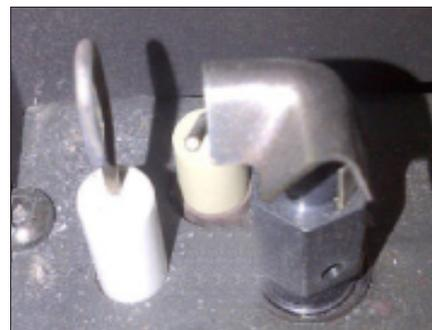
Figure 28 Proper Pilot Position
