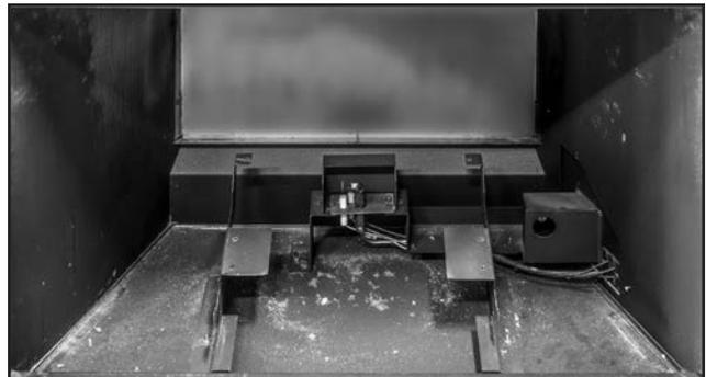
Figure 52: The rear liner can now be removed. Use a vacuum to clean up the bare firebox if needed.
