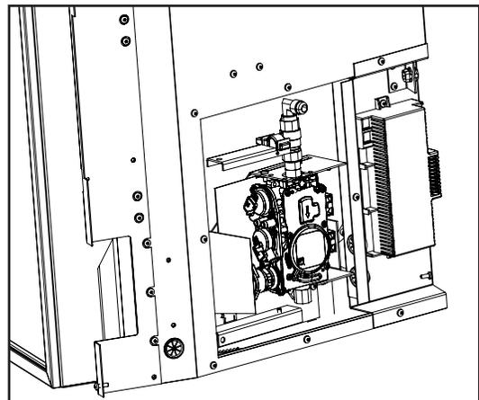
Figure 36: Gas valve with cover removed
