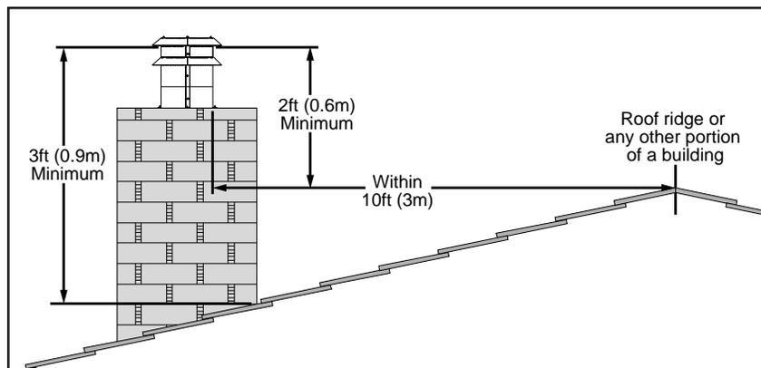
Figure 30: Roof Clearances.
