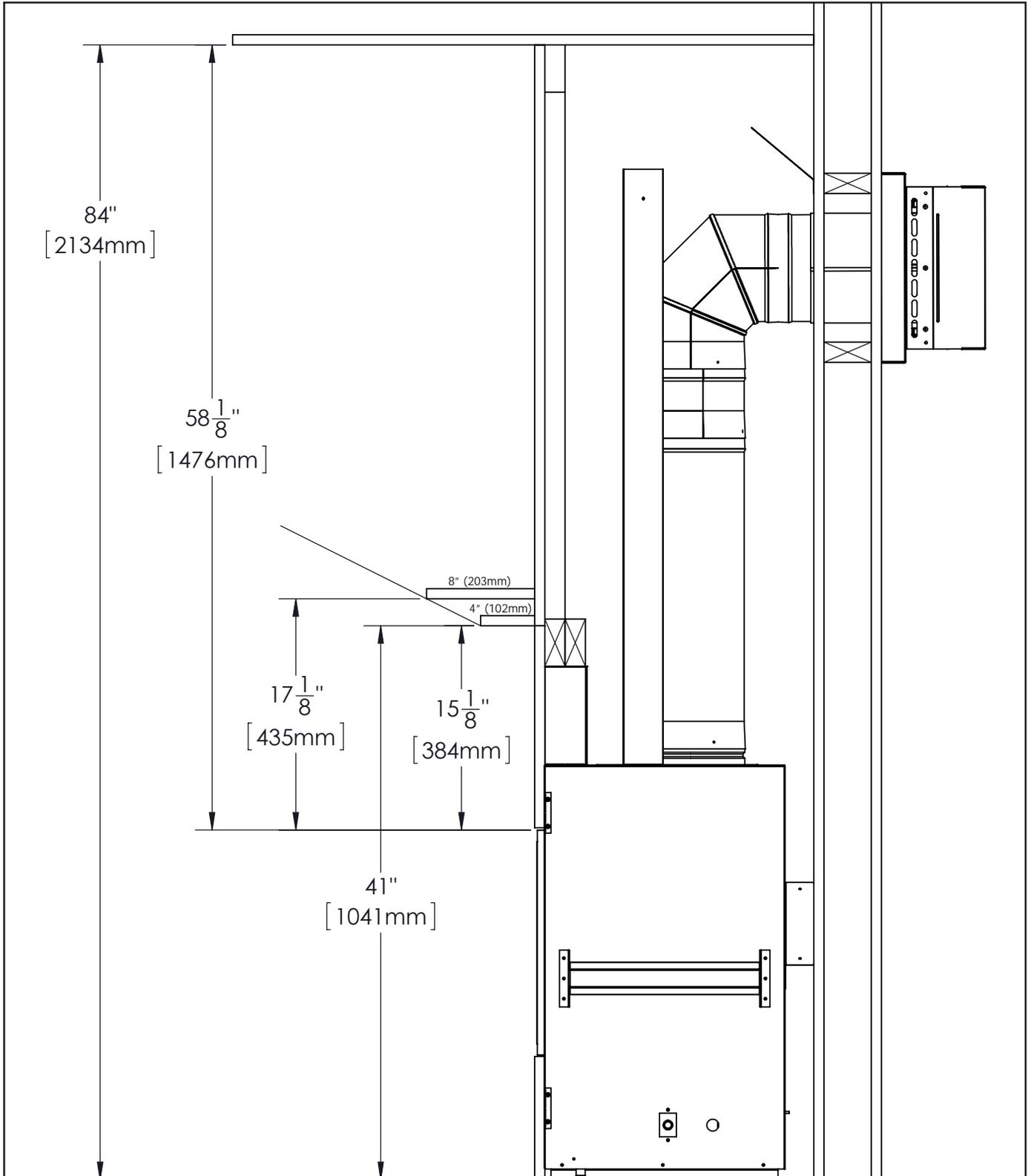
Figure 35: Install Dimensions with Mantel
