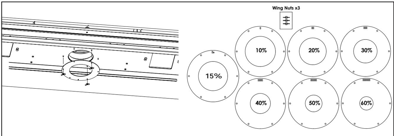
Figure 50: Restrictor Install and Ring Set
