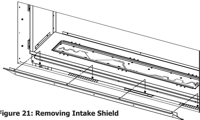
Figure 21: Removing Intake Shield
