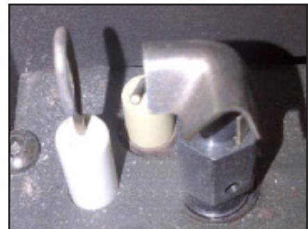
Figure 23: Proper Pilot Position
