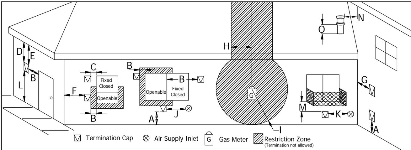
**Figure 47: Vent Termination Restrictions, refer to Table 3**
