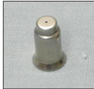
Figure 22: Pilot Orifice
