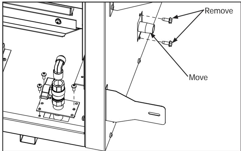
Figure 32: Alternate Gas Inlet Location
