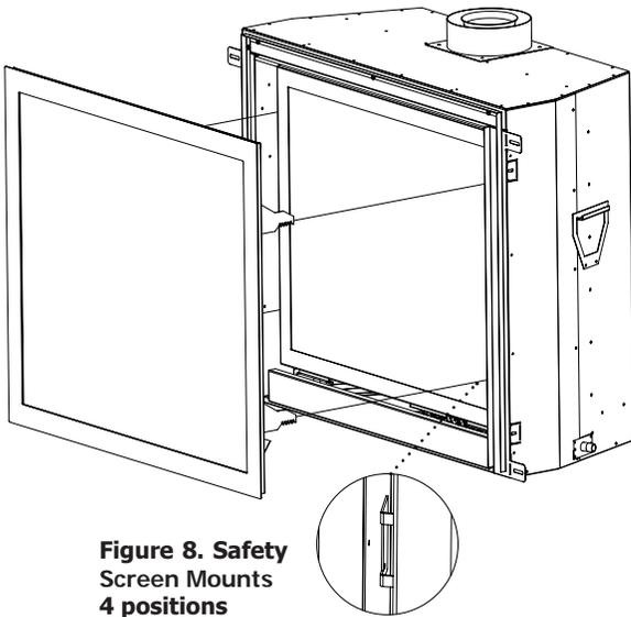
Figure 8. Safety Screen Mounts 4 positions
