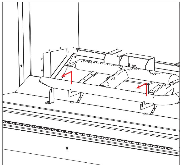
Figure 10. Removing Burner
