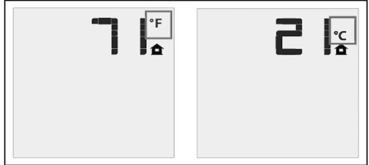
**Figure 8: Remote Control Display in Fahrenheit and Celsius.**
