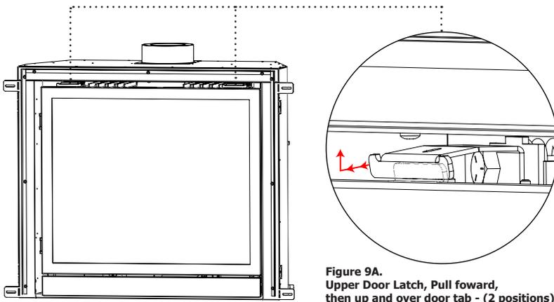
Figure 9A. Upper Door Latch, Pull forward, then up and over door tab - (2 positions)
