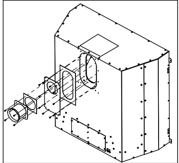
Figure 27b: Exhaust Block Off Plate Assembly Diagram
