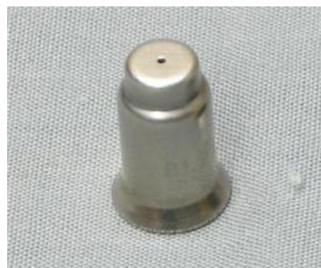
Figure 23. Pilot Orifice
