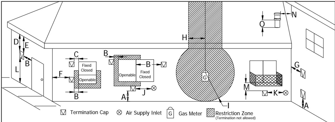
**Figure 33. Vent Termination Restrictions, refer to Table 4**
