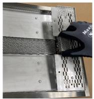
With the end sections of the media tray removed you grasp the remaining sections of the media tray and lift the burner assembly upward to remove it from the firebox.
