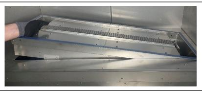
Reinstall the media tray cover and pilot shield and secure them to the appliance with the two screws removed in the first step.
