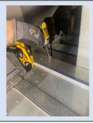
When all the panels are in place and secured, replace the (2) media tray end pieces and proceed with the firebox setup.
