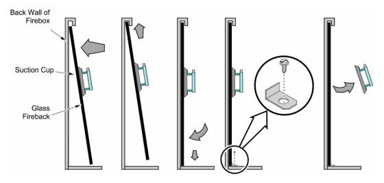
Install the left and right rear fireback sections first (single-sided only).
