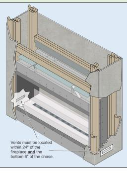
See-through unit chase must be vented on each end within 6" from the bottom of the chase (see left). Each vent must provide a minimum of <u>24 square inches</u> of free area.
