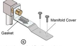
Apply thread sealant to the LP orifices prior to installation. Use the chart in the "Gas Specifications" section to determine the correct orifices.
