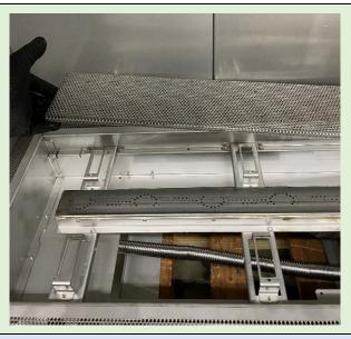
Remove the screws that secure the burner to the burner support brackets.
