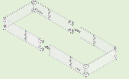
6. Put the (2) halves of the wind guard together and secure them by tightening the set screws on the center brackets. Make sure not to overtighten the screws.
