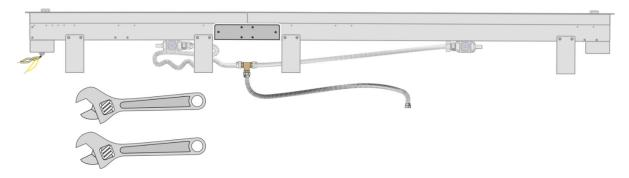
5. Connect the power from the 24VAC transformer to the two twisted pairs of wires that protrude from the end of side 1 of the appliance.
