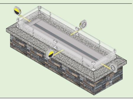
When all the clamps are secure use (2) people to lift the assembly and place it on the finish material around the Linear Fire Pit Burner. Measure the distance from the edges of the pit to the edges of the glass to ensure that it is centered.
