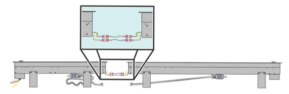
2. Once the wires are connected, slide the two halves of the fire pit together making sure not to pinch the wires between them.
