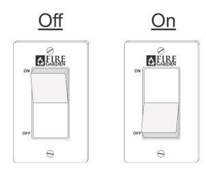
• If the wall switch will be located where it is not protected from precipitation, it must be installed in a weather resistant enclosure (not included).
