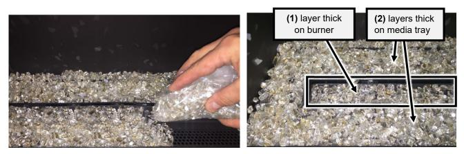
(b) Spread an even layer of crushed glass over the media tray and burner. The glass must be only (1) layer thick on the burner but can be (2) layers thick on the media tray. Excessive glass placed on the burner may cause poor burn characteristics and can lead to sooting and/or delayed ignitions.
