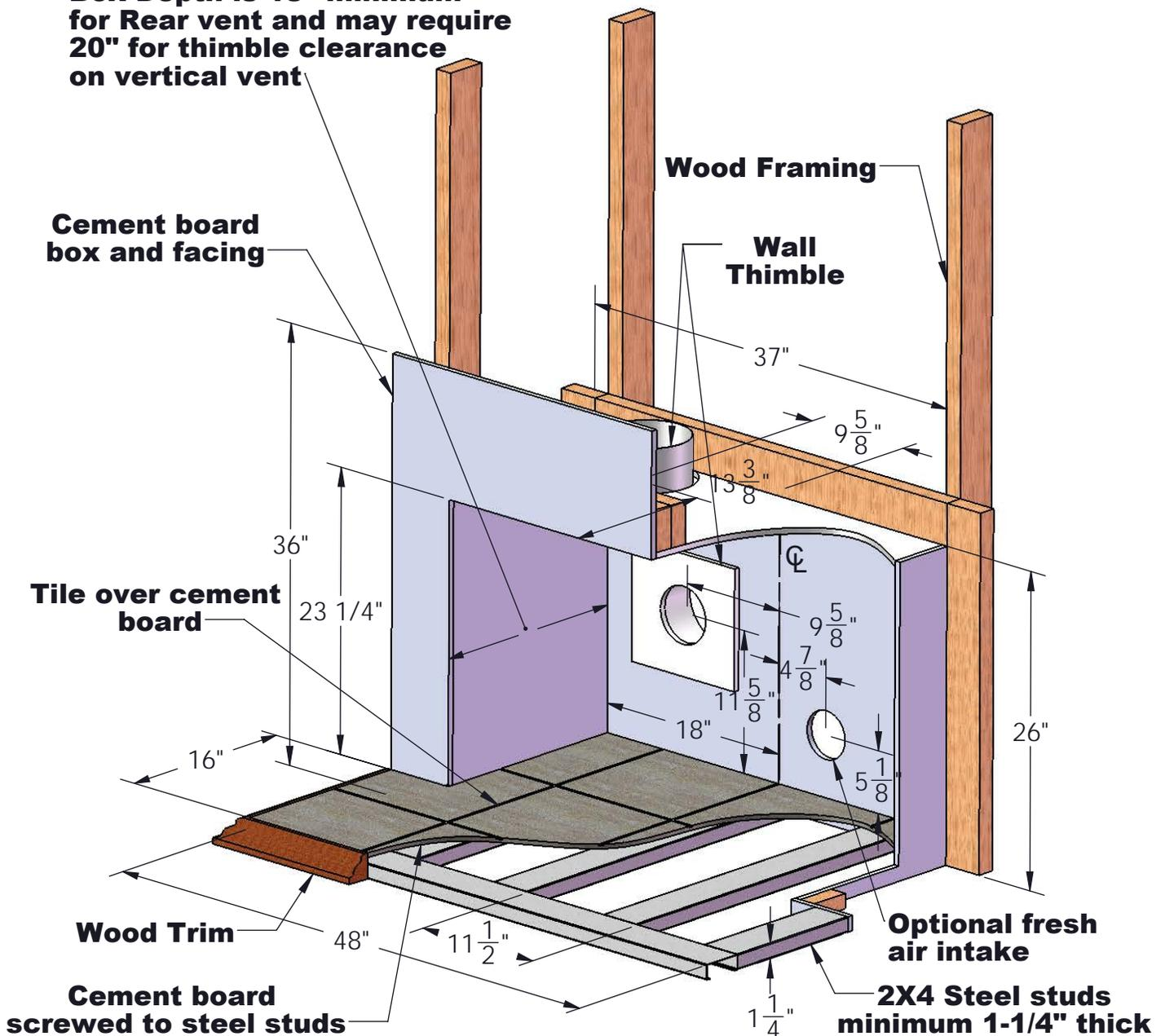
Figure 11: Built-In Specifications
