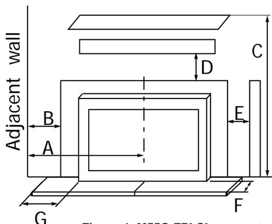
These dimensions are minimum clearances. It is recommended that you ensure sufficient room for servicing, routine cleaning and maintenance.
