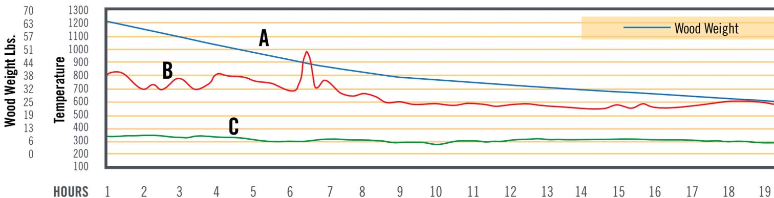
heat. The reduction in the weight of the wood load is greatest in the beginning as the moisture is boiled out of the wood. The blue line shows a very gradual & even reduction in the weight demonstrating the even heat output you can expect from a Blaze King catalytic wood stove.
