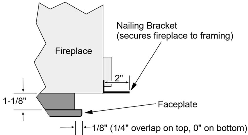
NOTE: Setup face is 1/16" wider on each side and top
