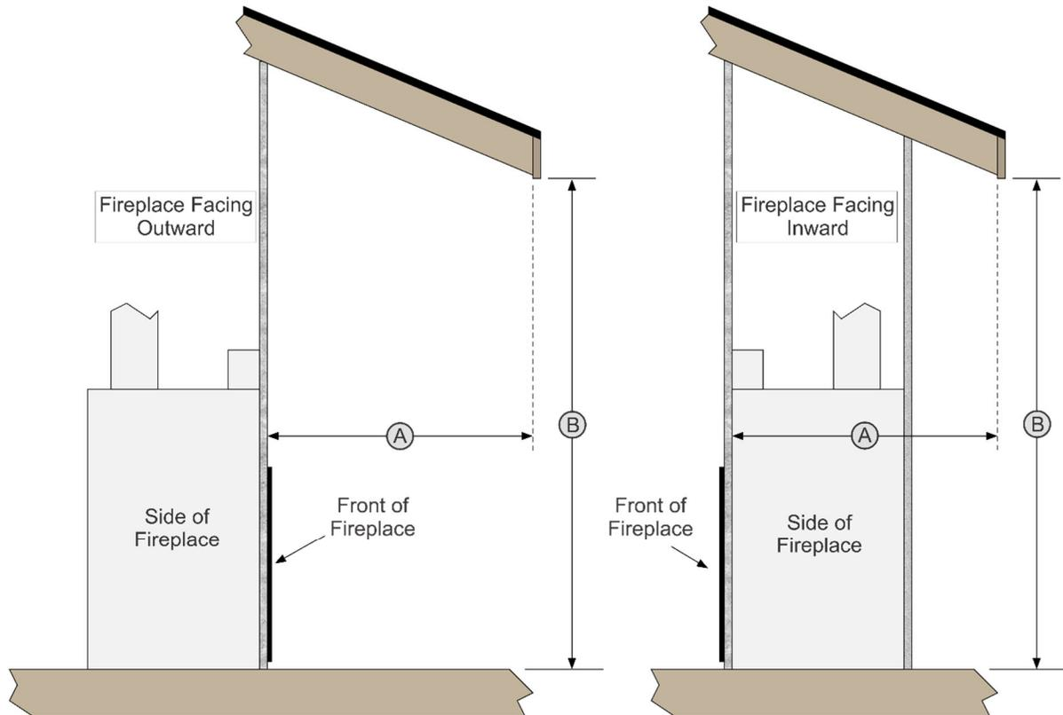
The overhang (A) must extend at least 1/2 the roofline height (B). Height is measured from the base of the fireplace.
