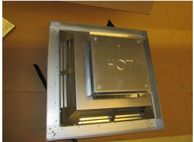
Attach the horizontal termination shield to the top of the horizontal termination as shown below (use the 4 included self-drilling screws). Note how the screws are installed from the top down.
