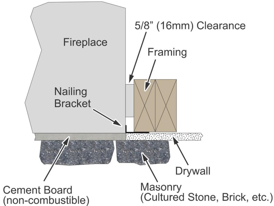
**Facing Example – Extended (Slab Over) Install**
