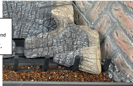
8. Place log #5 as shown below. There is a notch on the lower right of the log that rests against the leftmost fireplace grate finger. The upper portion of the log rests on a flat spot on the top of log #2.
