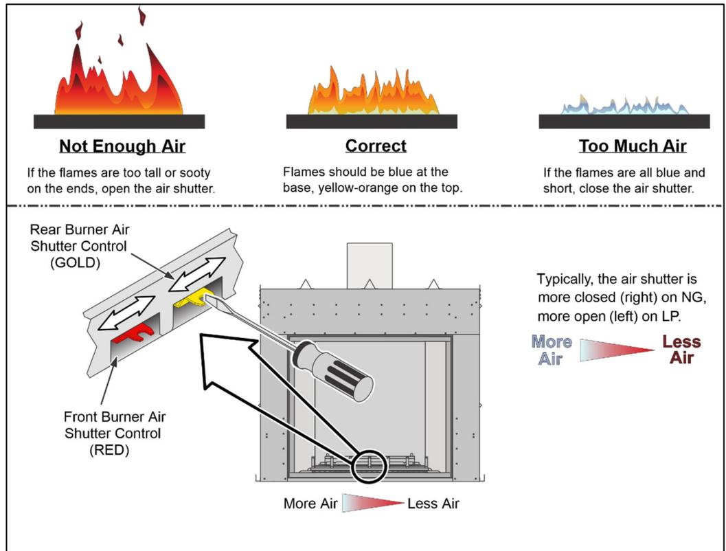
10. In manual mode on the remote, turn the flame height to the highest setting - the flames should not contact the top of the firebox. Check the flame on low position. The flames should burn off each burner hole. If the heater does not work correctly, contact your Travis dealer for assistance.
