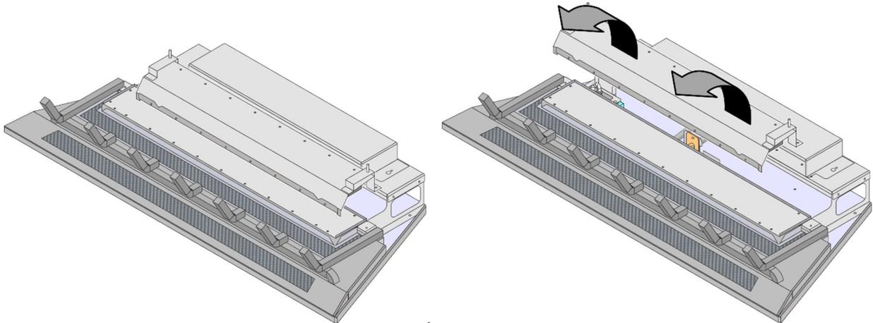
3. Remove the front burner. Lift up on the burner and remove it from the firebox (see below).
