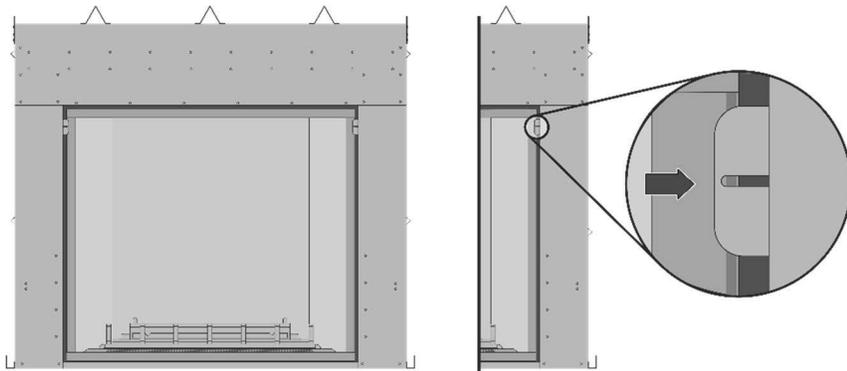
2. Use the glass latch tool to unlatch the glass frame on the two upper sides of the assembly. Tilt the top edge forward and lift to free the tabs on the bottom of the glass assembly out of the slots on the bottom of the fireplace opening. Remove the glass frame from the fireplace.
