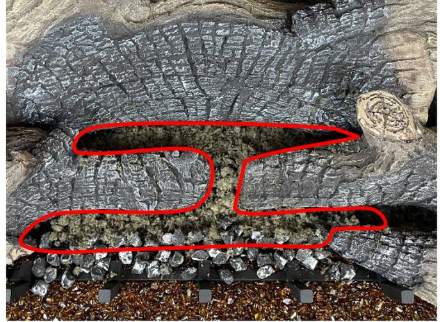
12. Place log #7 as shown below. There is a hole on the charred end of the log that rests on a locating pin on the right end of log #1 (see below). The other end of log #7 rests on the right end of log #3. Rotate the lower portion of the log until it is in contact with the fireback.
