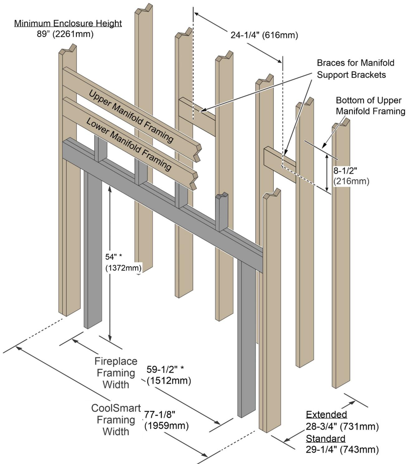
\* The dark-shaded framing should be installed after the fireplace is put into position. It is used to provide support for the facing above the fireplace and nailing brackets that secure the fireplace.
