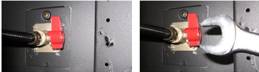
2. Remove the screw that holds the shutoff valve plate in place (1/4" nut driver). Remove the shutoff valve plate.
