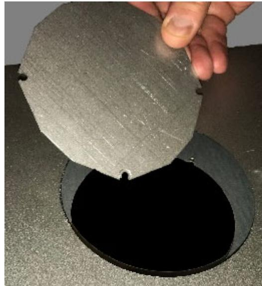
10 You will need to remove a third cover plate on each side. Remove the 2 screws holding the cover plate in place. Reach in and remove the cover plate. You may discard this plate.
