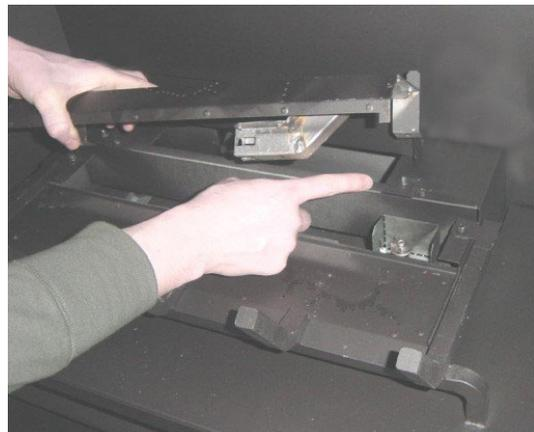
Lift the front burner, slide it to the right, and lift it from the firebox. When replacing the burner make sure it is properly located.
