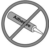
**WARNING:** Do not use adhesive, “modified thinset”, or any product with a polymer additive to secure facing directly to the fireplace or the walls near the fireplace. The high temperatures near the appliance will cause adhesives to emit odors. Use thinset (also called thinset mortar, thinset cement, dryset mortar, or drybond mortar) to attach the facing.
