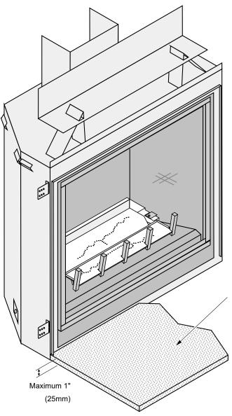
A hearth (combustible or noncombustible) may be installed in front of the fireplace. The structure must not extend more than 1" (25mm) above the base of the fireplace.
