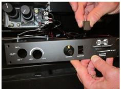
5 Remove the battery holder. Disconnect the red and black wire at the Molex connector.
