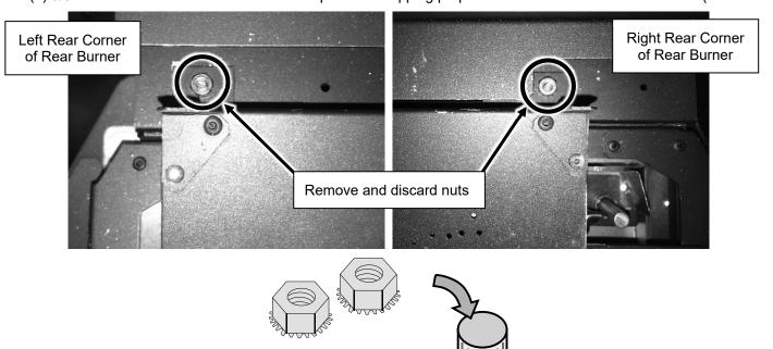
NOTE: Do not reinstall the shipping nuts. The burner brackets sit over the threaded pins and the burner needs to be able to move freely as it expands and contracts with heat.
