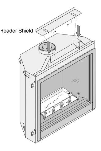
5 When finished the fireplace should be configured like the picture below.
