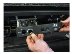
**NOTE** There should be enough slack in the attached wires to lower the dashboard to the floor. Make sure not to damage any of the attached wires.
