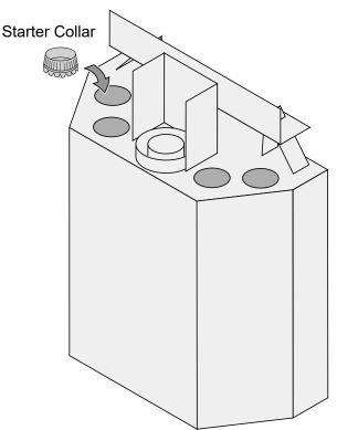
6 Install the fireplace into the framed chase. See section "Installation" in the manual.
