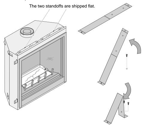
4. Attach the lower header shield to the header standoffs with 2 screws (see illustration below).
