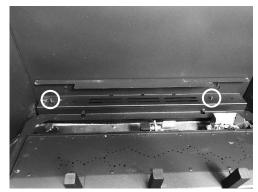
Lift the front burner, slide it to the right, and lift it from the firebox. When replacing the burner make sure it is properly located.
