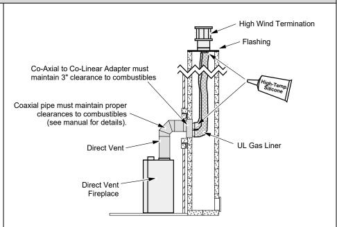
This appliance may utilize 6-5/8" diameter direct vent manufactured by Duravent (reducer may be required). The vent may be adapted to utilize an existing masonry fireplace using the Duravent Masonry Chimney Conversion Kit (part # 46DVA-KMC). The vent must be installed following all directions included with the vent and those listed below:
