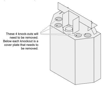
2 Use snips or diagonal cutters to snip the tab on the knockouts. Press on the far side away from the tap to pop the edge of the knockout up.
