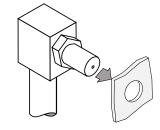
Adjustable Wrench 1/2" Open End Wrench Manifold Orifice
