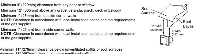
E Minimum 11" (279mm) clearance below unventilated soffits or roof surfaces Minimum 18" (457mm) clearance below ventilated soffits Minimum 6" (152mm) clearance below roof eaves NOTE: Vinyl surfaces require 24" (610mm) NOTE: Clearance in accordance with local installation codes and the requirements of the gas supplier.
