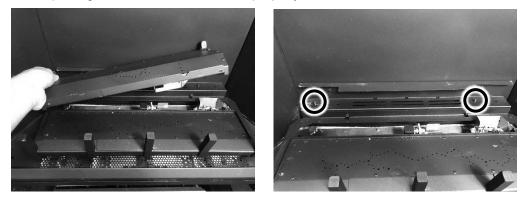
Lift the front burner, slide it to the right, and lift it from the firebox. When replacing the burner make sure it is properly located.
