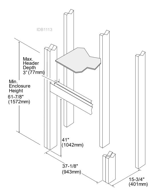
The fireplace enclosure must be a minimum 61-7/8" (1572mm) tall. Do not build into the fireplace enclosure.
