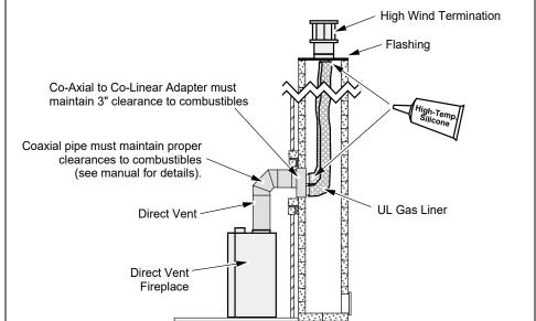
This appliance may utilize 6-5/8" diameter direct vent manufactured by Duravent (reducer may be required). The vent may be adapted to utilize an existing masonry fireplace using the Duravent Masonry Chimney Conversion Kit (part # 46DVA-KMC). The vent must be installed following all directions included with the vent and those listed below:
