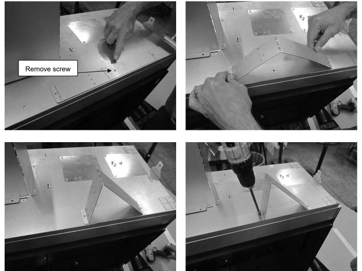
4 On the header shield, bend the two tabs downward approximately 90 degrees. Set the header shield onto the standoffs with the 90° bend facing the pipe shield. The tips of the standoffs will protrude through the heat shield. Attach the heat shield to the standoffs by aligning the holes on the heat shield tabs with the holes in the header standoffs and secure using the included screws
