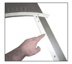
Attach the side gaskets in the same fashion, making sure the holes in the gasket line up with the holes on the face.
