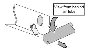
Pivot the air tube downwards and slide it out of the air channel on the opposite side.
