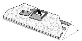
10. Remove the slide plate from the insert (see below).
