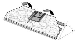
8. Lift the yoke out of the cups on the bypass damper and remove it from the insert (see below).
