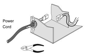
Re-attach the strain relief to the left side (use pliers to compress the strain relief from the top and bottom while pushing it into the hole).
