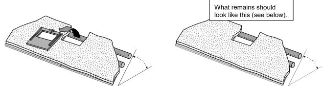
11. The illustration below shows what the front edge of the baffle should look like. Notice the baffle board is made of two separate pieces and there is a ceramic fiber blanket laying on both pieces of board. Grab both pieces of the baffle board and slide them together so that they overlap 2" to 4", this will make the baffle small enough to remove from the unit
