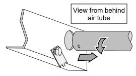
The pin will then disengage from the air tube (you may wish to rotate the tube slightly).
