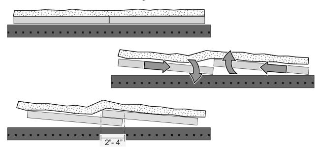
12. With the baffle board overlapping each other, both baffle board pieces and the blanket should now fit through the insert door opening.
