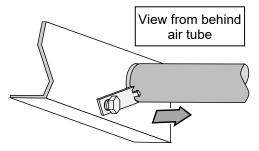
With the bolt loosened the air tube can be slid out of the air channel.
