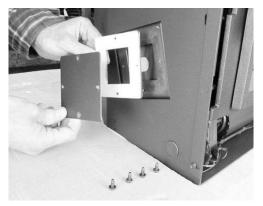
5. Install the housing as shown below. NOTE: The gasket's hole patterns are unique. The housing must be re-installed in the same configuration. If the holes are not aligned, rotate the gasket 90°.
