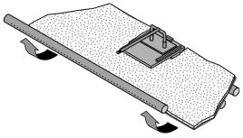
7. Lower the font edge of the baffle to gain access to the yoke and bypass components. Continue supporting the front edge of the baffle.
