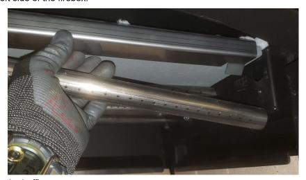
4 Remove the baffle cap.
