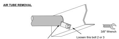
Note how the center of the air tube pin turns (do not remove). inserts into a hole on the air tube.
