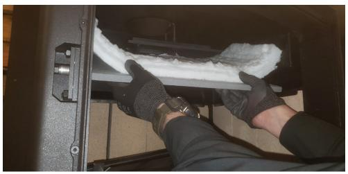
8 Tilt the baffle and blanket to allow them to pass through the door opening and remove them from the firebox.
