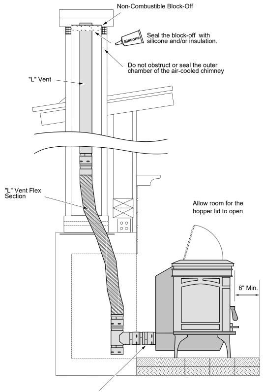
NOTE: you may need a short horizontal section here to clear the lintel and allow the hopper lid to open.
