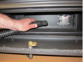
3. Remove the access plate on the exhaust blower housing by removing the (6) 1/4" hex head screws. Remove the plate and gasket and keep these parts for reinstallation. If the gasket material is deteriorated or damaged replace it when reinstalling the cover plate. Clean the combustion blower with the bottle brush or vacuum.
