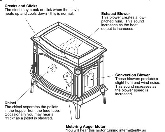
it feeds pellets. You may also hear the pellets drop into the feed tube.
