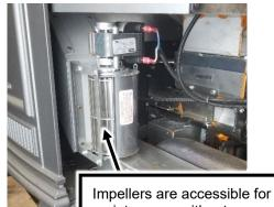
Impellers are accessible for maintenance without removing blower.
