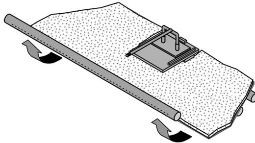
7. Lower the front edge of the baffle to gain access to the yoke and bypass components. Continue supporting the front edge of the baffle.
