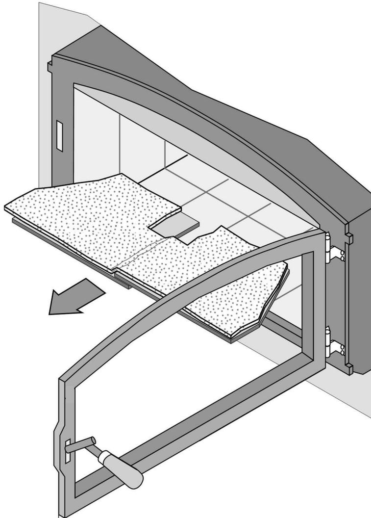
**NOTE:** To reassemble the baffle, follow the steps above in reverse.
