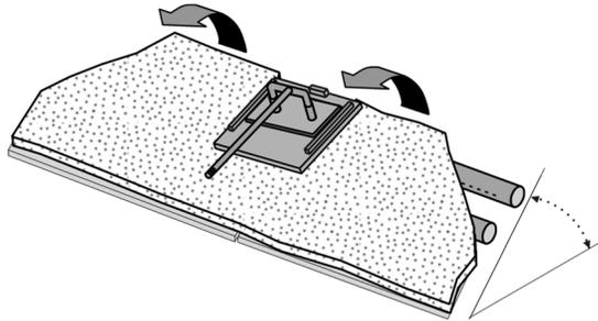
8. Lift the yoke out of the cups on the bypass damper and remove it from the insert (see below).
