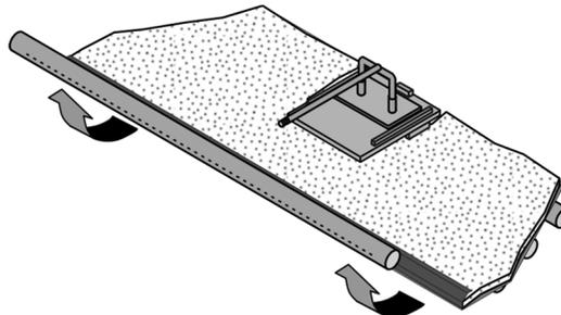
5. Remove the Baffle Cap from the front edge of the baffle board and blanket (see below).
