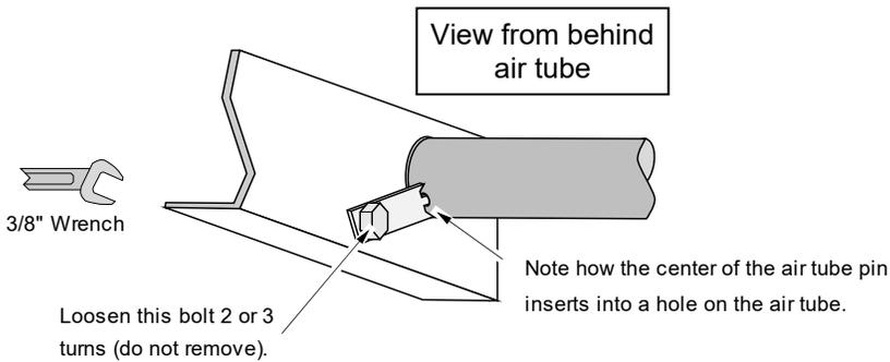
Loosen this bolt 2 or 3 turns (do not remove).
