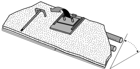
9. Lift the bypass damper off the slide plate and remove it from the insert (see below).
