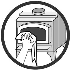
Maintain the door and glass seal and keep them in good condition. Do not operate this heater with broken or missing glass. Avoid placing wood against the glass when loading. Do not slam the door or strike the glass.
