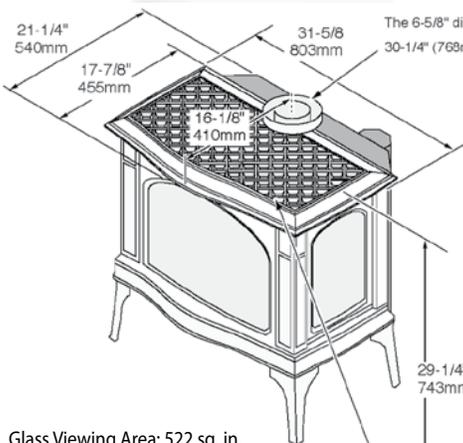
The 6-5/8" diameter flue collar is 30-1/4" (768mm) above the floor
