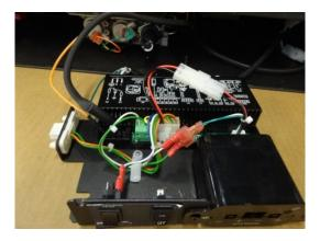
9 Remove the switch from the bracket and replace it with the blank that is included with this kit. To remove the switch squeeze the tabs on the top and bottom of the switch while pushing on the back side of the switch.
