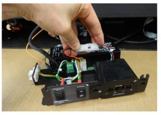
8 Remove the green and white wires from the back of the burner ON/OFF switch and attach them to the green and white wires coming from the back of the receiver. <u>Make sure the green wire is to the green wire and the white wire is to the white wire.</u>
