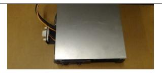
4 Loosen the two screws that hold the heat shield on the Electronic Controls Assembly and lift the front of the heatshield until you can disengage the rear leg of the heat shield from the back of the Electronic Controls Assembly. Slide the grommet, holding the pilot wires,out of the rear leg on the heat shield. Remove the heat shield and set it aside for reinstallation.
