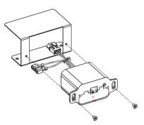
7 Install and screw the receiver to the Electronic Controls Assembly housing using the two Philips head screws that were removed in the previous step. Connect the Molex connector from the receiver to the Molex connector disconnected in the previous step.
