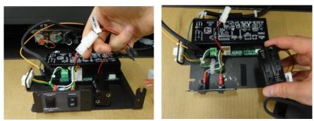
6 Remove the receiver from the mounting bracket. Use the two screws in the following step. Discard the mounting bracket.
