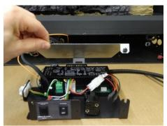
5 Disconnect the red and black wires that attach to the battery holder by separating the white Molex connector as shown below. Once the wires are disconnected, remove and discard the battery holder which is held in place with hook and loop tape.
