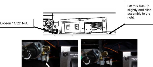
This connection will disengage as the assembly moves right. The assembly can then be removed as shown below.
