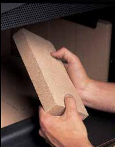
Lopi uses real kiln-fired, refractory firebrick in the firebox. This is the same material used to line commercial boilers and furnaces, and is twice the weight of typical brick. The brick protects the steel while increasing the internal temperature within the firebox.
