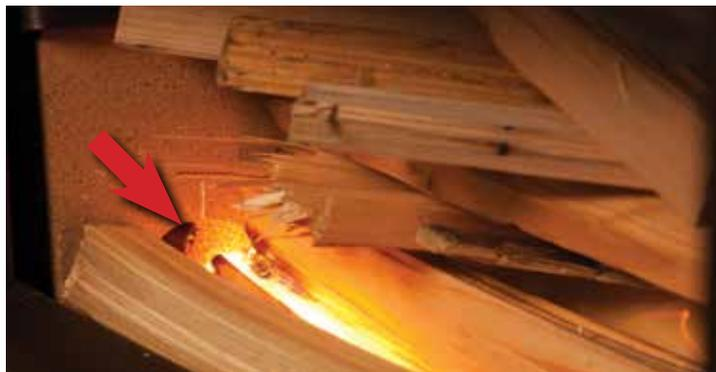
**2** A compressor will force 1,400 degree preheated air into the firebox directly onto the wood, giving a clean, fast, smoke-free start up within 30 seconds.
