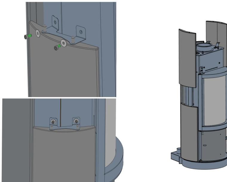
10. Align the top body securing brackets with the holes in the top stone panel, adjust the stone panels up and down by removing or adding washers to the threaded studs on the body bottom. Once adjusted, tighten the screws to lock the stone panel in place.
