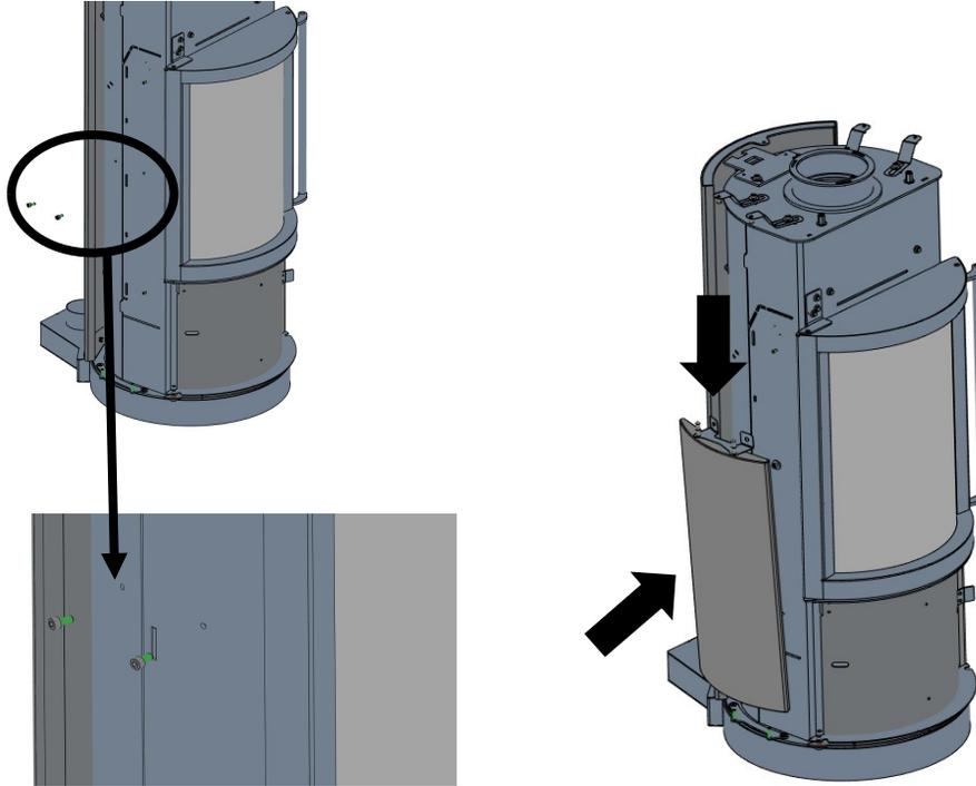
9. Once the lower side stone panel is installed, reinstall the previously removed screws to secure the soapstone panel bracket to the body of the stove. Install the top soapstone panels to the lower panel's top bracket by aligning the panel's bottom holes to the silicone sleeves, and firmly press the stone down onto the bracket.
