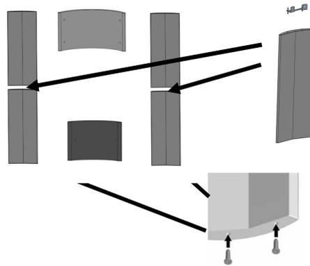
4. Remove the threaded studs and hex nuts from the Bari base where the sides will go.
