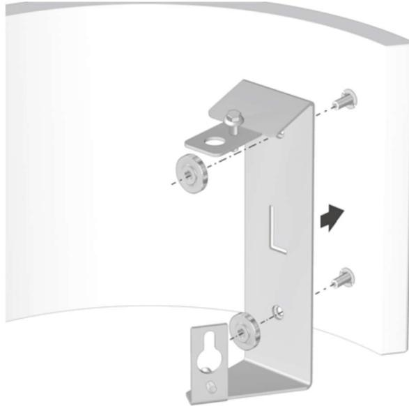
9. Repeat this procedure with the right bracket T09 on the left side of the front top stone panel.
