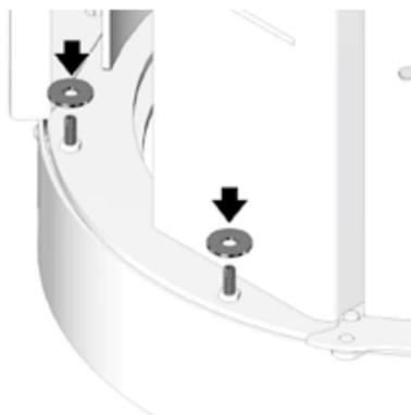
3. **For Ceramic Panels:** Align each side's bottom holes onto the bottom side studs and push the side firmly down so the threaded studs engage the mounting holes.
