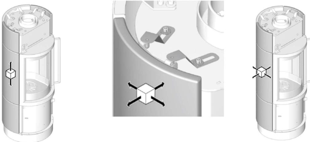
6. Tighten top body bracket screws to lock the sides in place once the adjustments are properly made and the sides have an even panel gap and height with the back panel.
