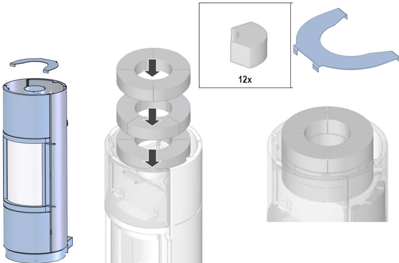
21. **For Bari Plus 8172 units:** Install the leveling hardware to the indicated height. Attach the top to the body of the stove and ensure a slight gap between the top and stove body.
