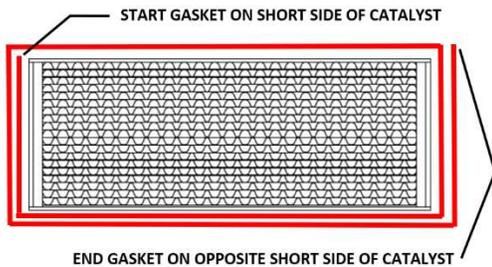
9. Beginning at one corner, re-install fiberglass gasket material on the catalysts.
