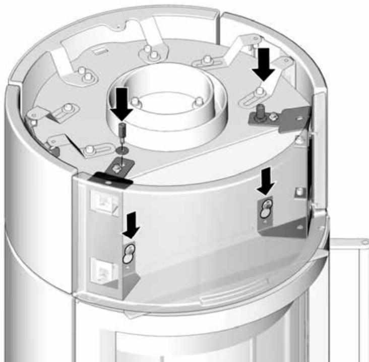
15. Adjust the front top panel until it is flush vertically and horizontally with the other body panels.
