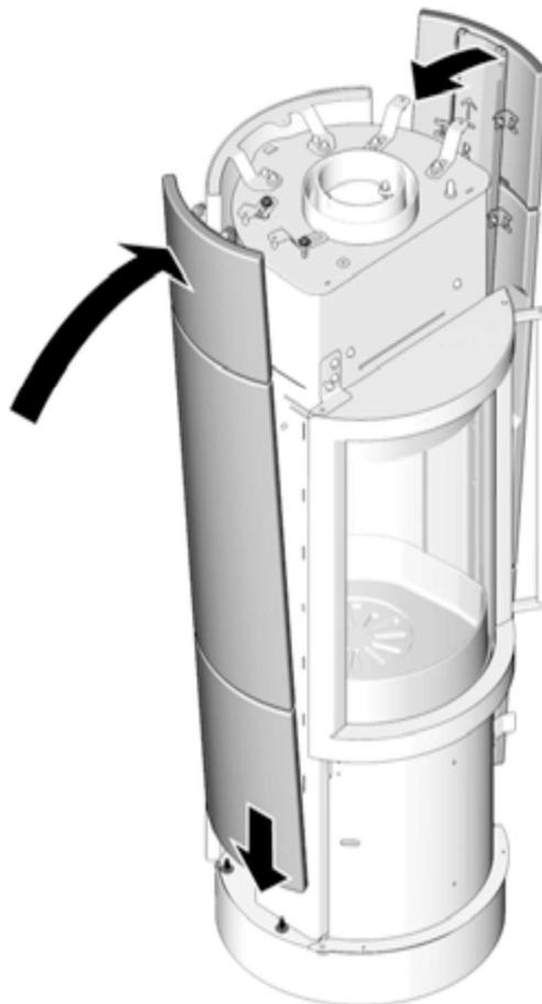
4. Align the threaded studs on the top body brackets into each side's top panel bracket.
