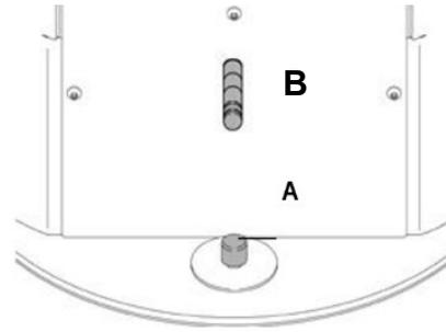
**ROTATION CONTROL:** Your Bari rotates a full 180 degrees. With the stove centered on your hearth, it will rotate 90 degrees to the left and 90 degrees to the right.
