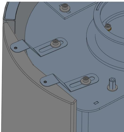
11. **For Both Soapstone and Ceramic body kits:** Remove the thumb nuts from the lower front body panel. Align the threaded inserts on the panel with the holes in the lower front door. Reinstall thumb nuts to secure lower panel to the lower front door.
