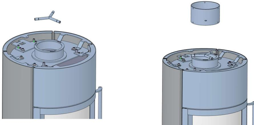
5. Install the provided screws and washers into the threaded holes of the top section of the flue collar to secure the flue collar in place. The screws should hook under the lip of the lower flue collar and allow the flue collar to rotate freely.
