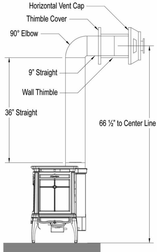
**Figure 10 - Typical Minimum Horizontal Venting Installation Components**
