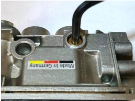
Figure 21 – Low Flow Orifice Removal
