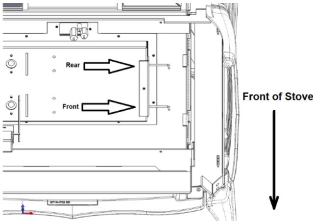
**Figure 38 – Stove Bottom View: Air Shutter Adjusting Rods**
