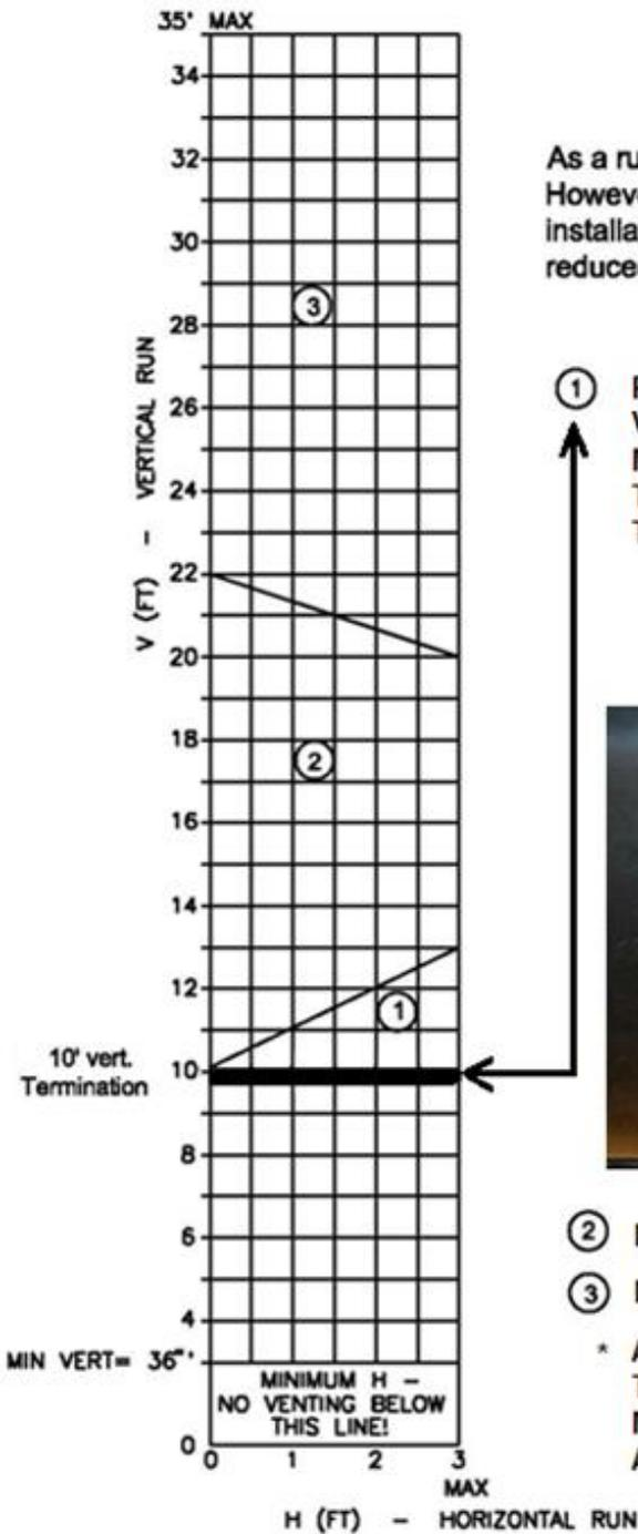
As a rule, only two 90 degree elbows are allowable. However if more than two are **required** to complete the installation, the maximum allowable vent length must be reduced by 5' for each additional elbow.
