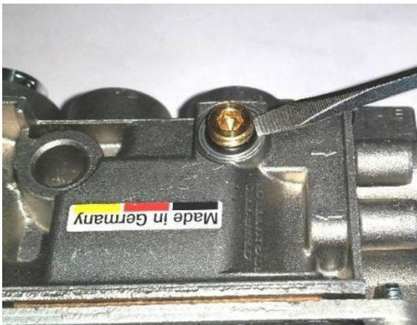
Figure 22 – Low Flow Orifice Removal – O-ring
