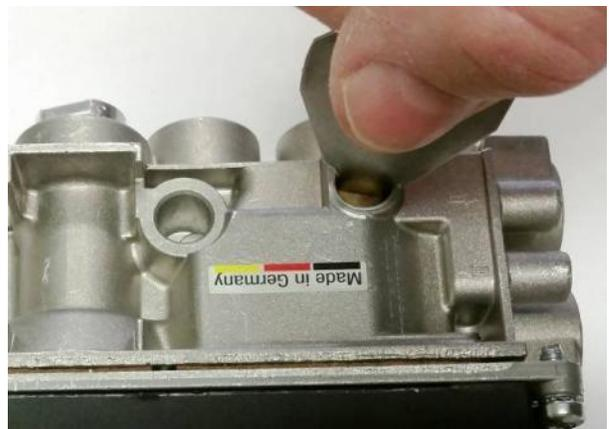
Figure 25 – Tighten LP Low Flow Orifice
