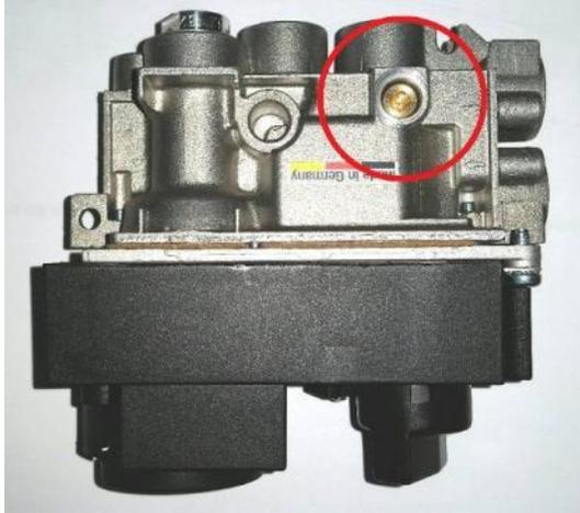
Figure 20 – Low Flow Orifice Location
