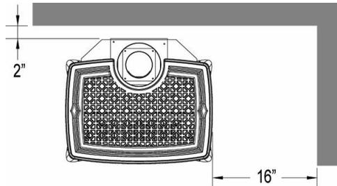
Figure 5 - Minimum Wall Clearances
