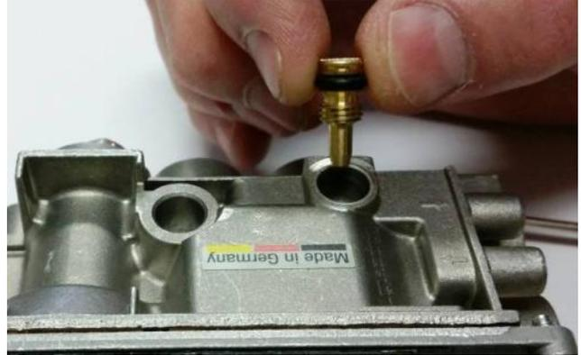
Figure 23 – NG Low Flow Screw Removal
