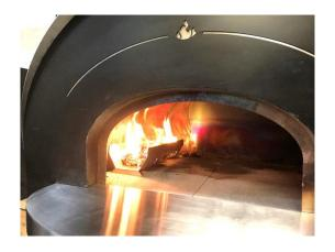
Light the paper. Put the door on the unit, but leave the door spaced out 2" from the front of the unit while the fire gets started. This will allow for oxygen to feed the fire, and will prevent smoke from coming out of the door while the flame is established.
